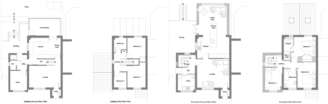
The angled outline top right of each floor plan represents the neighbour's conservatory
