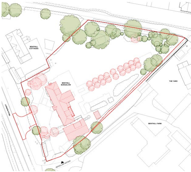
Existing site plan with buildings and 28 trees to be removed in red
