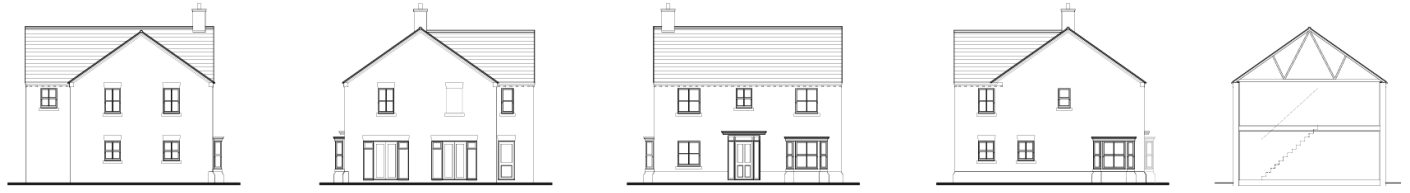
Existing rear (facing SE) side facing SW front facing NW side facing NE section The window outlined on the SW-facing elevation would have served the Bedroom 2 en-suite bathroom but does not feature on the floorplan below, so is not a drawing error.
