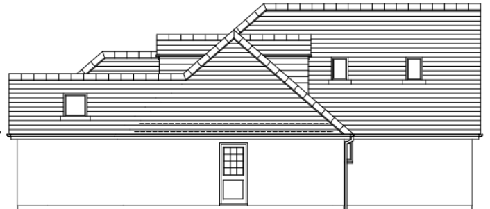
Proposed side elevation facing No 132. The floor plan only shows one skylight in the new roof.
