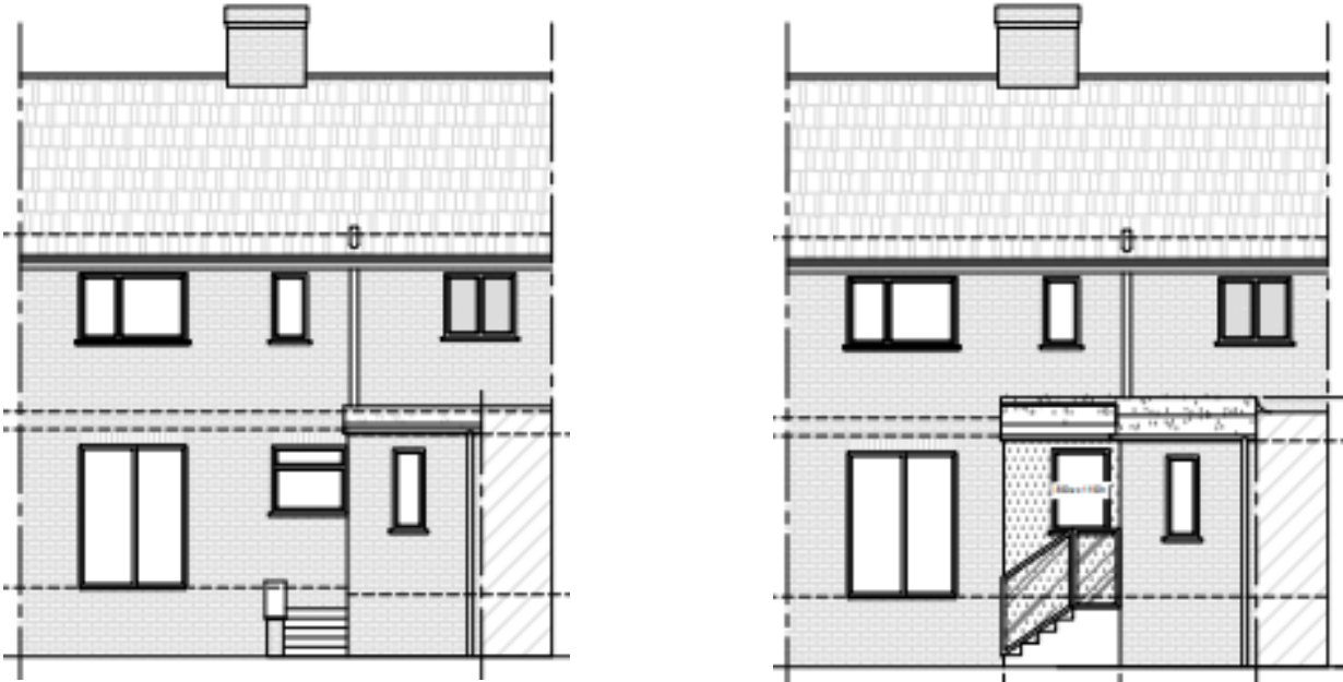
Existing and proposed rear elevation (lowest dashed line is front elevation ground level)
