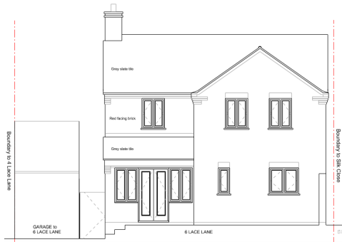
Existing rear elevation
