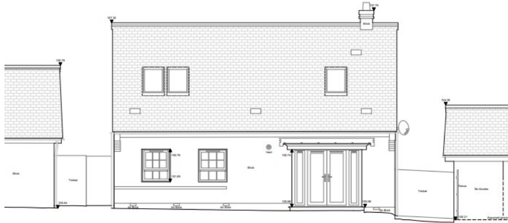
Existing rear elevation and neighbouring garages
