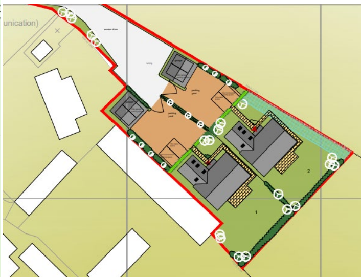
Proposed site plan; the blue-green strip along the Lace Hill fence shows the easement for the septic tank
