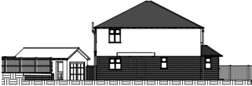
Proposed north side elevation; deleted door is in the kitchen New windows both to new kitchen areas
