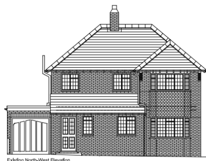
Existing front elevation
