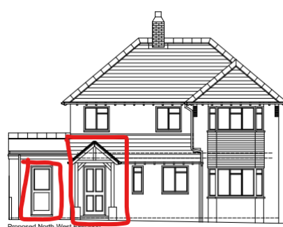
New door and porch
