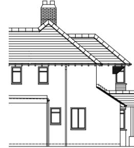
revised side extension and porch The new window is onto the hall
