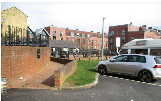
The new disabled parking bays are convenient for the ramp which leads to the ground floor level of the hotel (see drawing on p14). However they are at right angles to the kerb, which makes the shape of bay 5 problematical, especially as it isn't regulation width.
