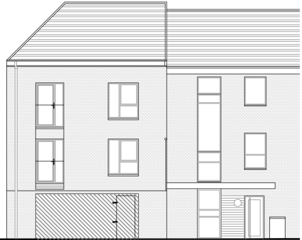
Existing front (south) elevation
