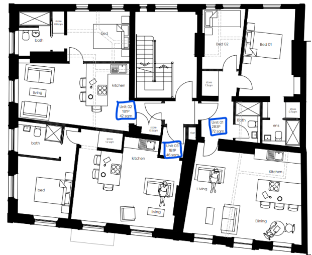
Proposed 1st floor – 1 x 2-bed and 2 x 1-bed flats
