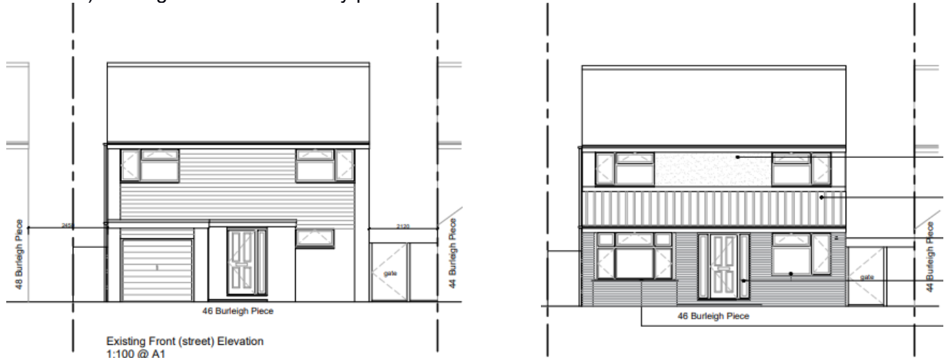
Existing and Proposed front (street) elevations
