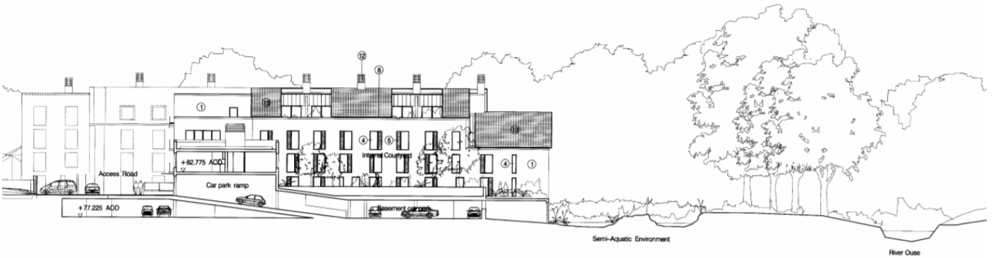
Section through the site between this block and the central one (their floor levels are the same) 2007 application
