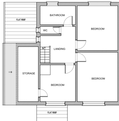
Existing first floor layout
