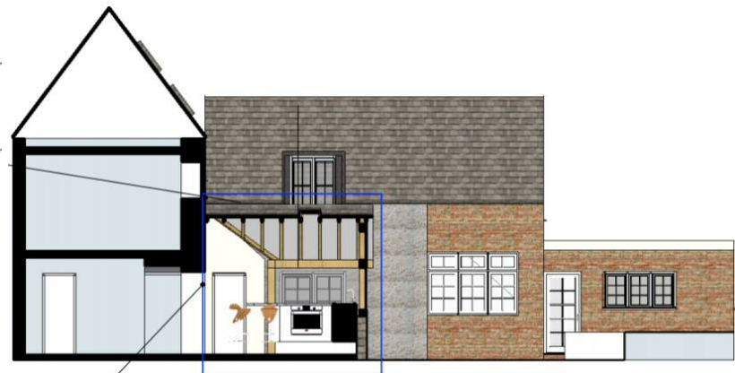
Proposed rear elevation and section (blue line shows new extension) Existing roofline is maintained.
