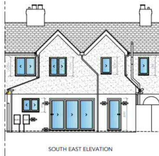
Existing and proposed rear elevations; the new single-pane windows at first floor level will be obscure-glazed
