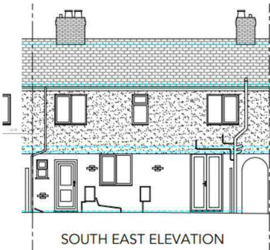
Existing and proposed rear elevations; the new single-pane windows at first floor level will be obscure-glazed
