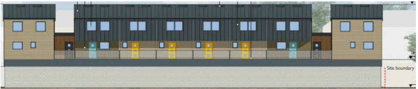
Original rear elevation drawing; Rooflights shown as black line near roof ridge
