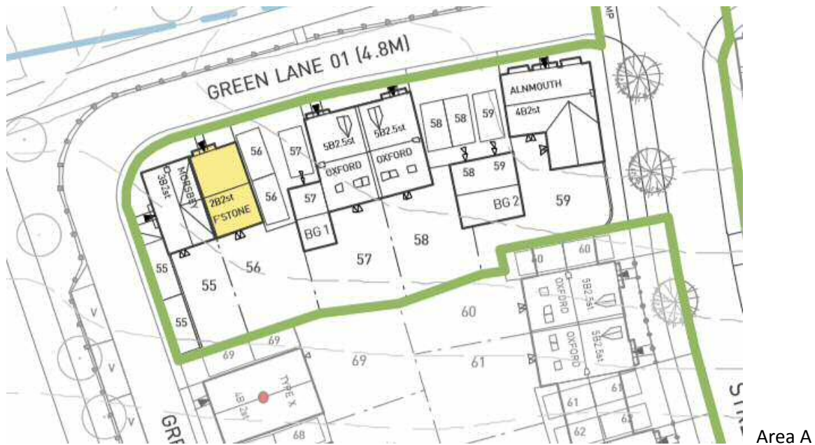
(A). Additional unit inserted. Alderney (4-bed) house type replaced with a Morseby (3-bed) & Folkestone (2-bed) on plots 55 & 56.
