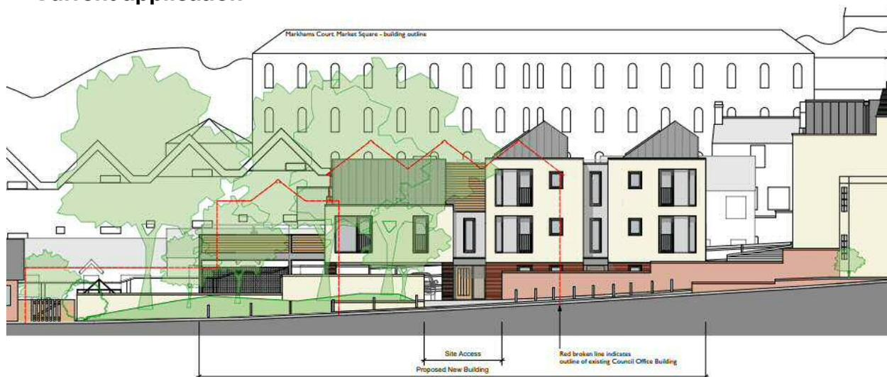
Verney Close elevation, with trees and adjacent buildings. The red outline shows the roof profile of the Buckingham Centre for height comparison. There is no comparable perspective view with this submission.
